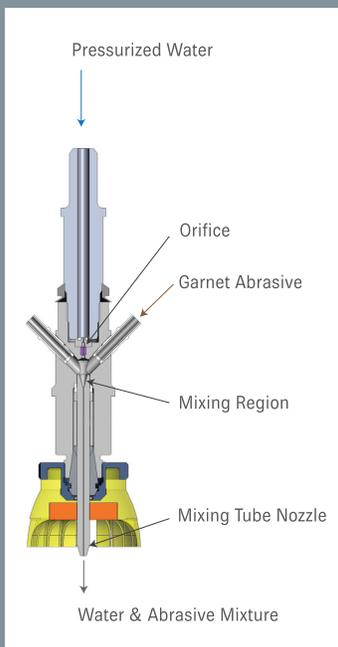
from very low velocity via a venturi effect (a way of creating suction) and then accelerated down the mixing tube by the supersonic water (Figure 4). Therefore, the abrasive speed is governed by the water speed. As Dr. Hashish says, "Increasing power by increasing the pressure and not the flow rate gives us the benefit of increased velocity."
