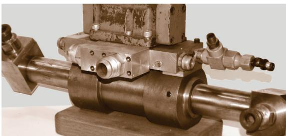
Flow's first commercial waterjet intensifier at 30,000 psi, 1972
